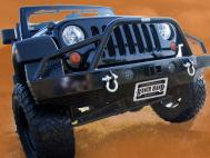
Jeep Bullnose" fully welded formed channel 1 piece design comes standard with a built in 2" receiver, shackle bracket mounts, and durable powder coat finish. **Optional Winch Plate for mounting** a number of Warn winches: XD9000, 9.5ti, 9.5si, and the Powerplant HP.
