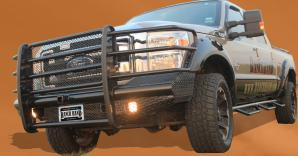
"Legend Front End Replacement" known for its legendary quality is manufactured with 4" Schedule 40 Pipe and provides maximum protection for your vehicle. It is designed to take an impact both on and off the road and comes standard with a 2" receiver. Field tested in extreme conditions, this is the toughest product on the market today. Most applications retain factory fog lights and tow hooks.
